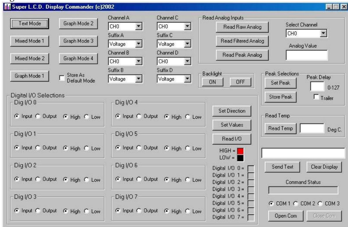
**Communicating:** To start the communication between the PC and the L.C.D. select the COM Port that the module was connected to in “**Connecting Hardware:**” and click the *Open Com* button. After communication has been established, clicking any button on the interface except *Send Text* or *Clear Display* will turn the Command Status indicator
